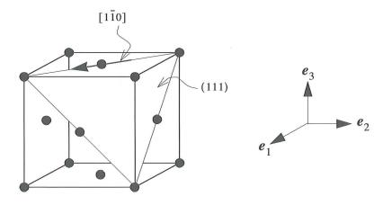
In terms of components with respect to the orthonormal basis  $\{e_i\}$  (i = 1, 2, 3) this  $(111)[1\bar{1}0]$  slip system is characterized by the slip plane normal vector  $\mathbf{m}$  and slip direction  $\mathbf{s}$  given as  $\mathbf{l}$
