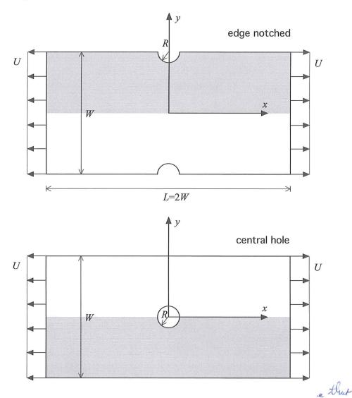
The total amount of material left is the same, and in fact the gray areas indicating symmetric halves are identical. Nevertheless, the two plates will respond to an applied displacement U in different ways (even if they have the same uniform material properties). Apparently something in the entire set of governing equations is different; the question is: what? Support your explanation with mathematical statements.
